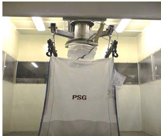
FIGURE 5: BIG-BAG FILLING HEAD
