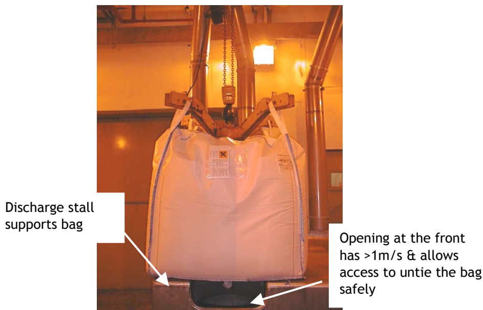
FIGURE 2: ENZYME BAG DISCHARGE
